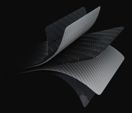
This groundbreaking application has led to a remarkable 300% increase in strength compared to the conventional polyester-glass laminate as well as 30% reduction in the boat's overall weight.
